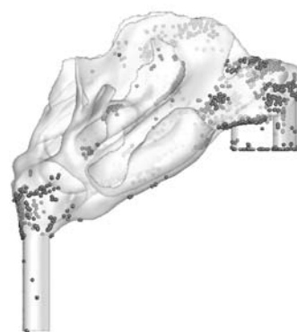
Figure 2. Particle deposition characteristics on the wall of the nasal cavity.
